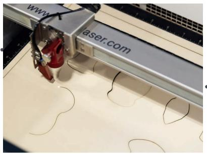
Cut the shapes with the laser cutter
